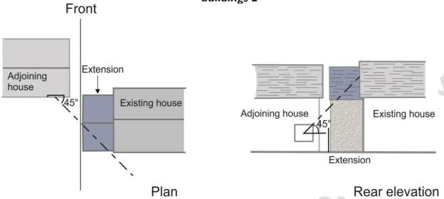
The extension at the neighbouring property breaches a 45 degree <u>angle line</u> both in plan and elevation\_<u>drawn from the window of a habitable room in the neighbouring property.</u>
